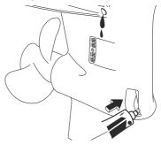
(9) Put a new gasket on the oil level plug. When the gear oil begins to flow out of the oil level plug hole, insert and tighten the oil level plug to the specified torque.
