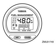
To change the fuel flow display, press the "set" (set) button repeatedly until the gauge displays "S" (for fuel flow to the starboard engine only), "P" (for fuel flow to the port engine only), or "P S" (for total fuel flow both engines).
